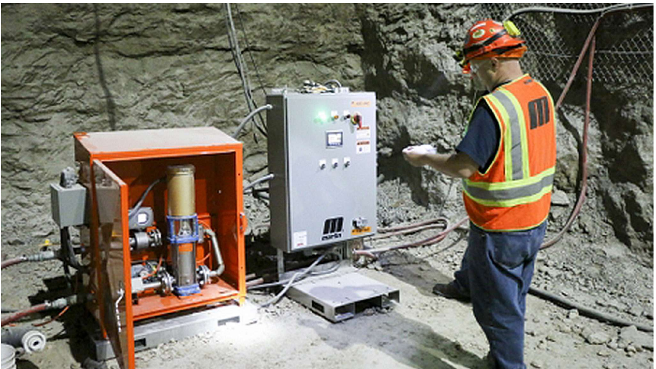
Monitors, valves and boosters are set in accessible cabinets so the system is easy to inspect and maintain.
