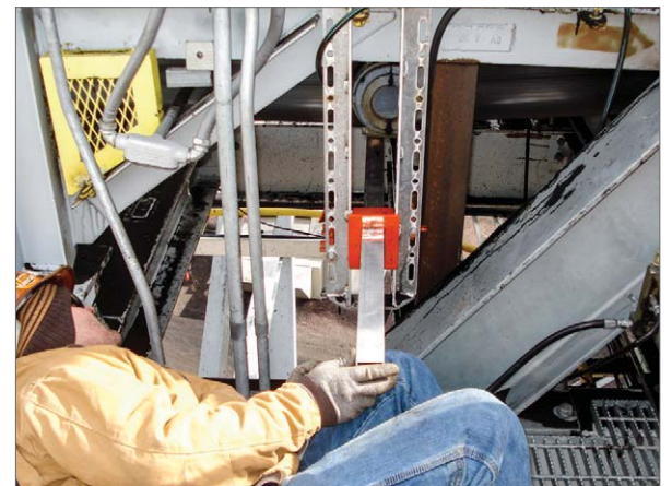
The Martin conveyor belt carryback gauge is a patented tool for estimating carryback on the return side of a conveyor belt.
