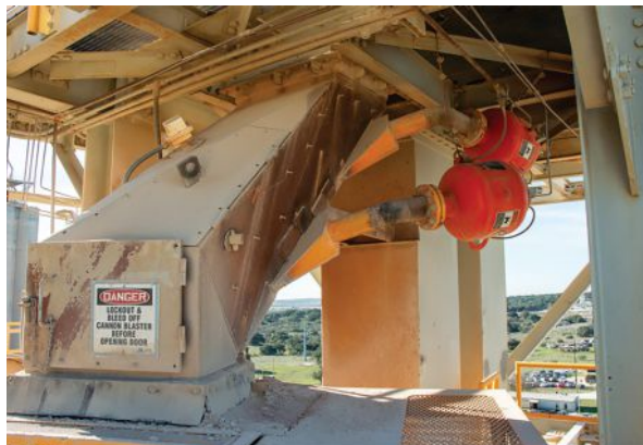
Air cannons can dislodge material and prevent buildup by distributing powerful shots of air inside a vessel.
