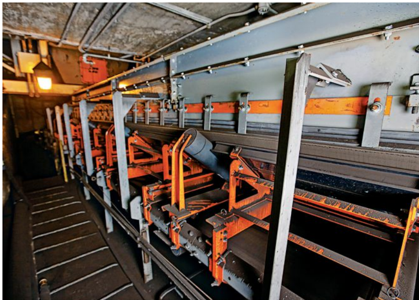
Inspection doors and track-mounted components facilitate maintenance for extended equipment life.
