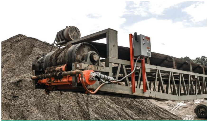
New designs can even control belt tensioning and pull the blade away from an unloaded belt.
