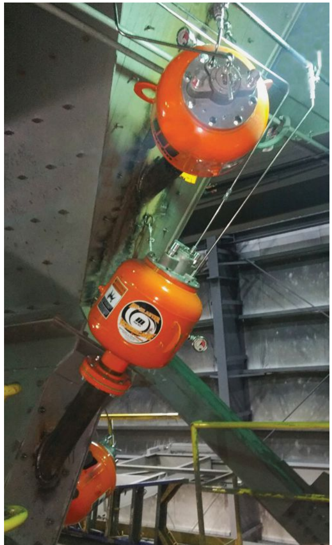
Safety cables secure the cannons to the vessel.
