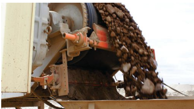
Properly positioned and tensioned primary and secondary cleaners mitigate belt wear issues commonly associated with cleaners. Photo: Martin Engineering
