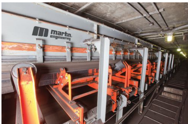
Properly positioned and tensioned primary and secondary cleaners mitigate belt wear issues commonly associated with cleaners. Photo: Martin Engineering
