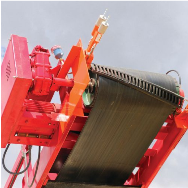
Innovative cleaner design reduces belt wear and eliminates the need for re-tensioning. Photo: Martin Engineering
