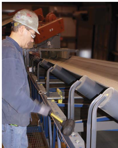
"Knocking" an idler with a mallet to change its position.
