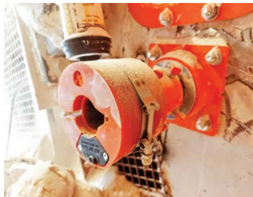
Above: Service teams can use remote monitoring data to visit the belt cleaner blades most in need of attention.
