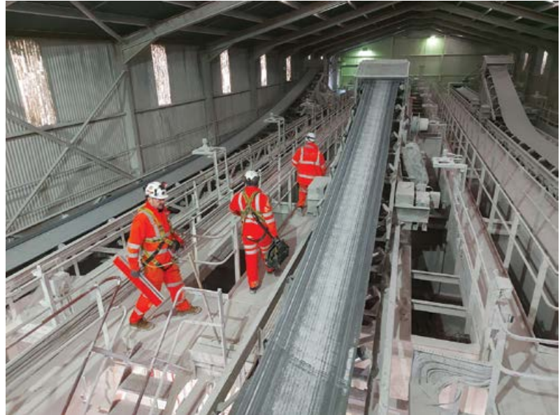
Above: Service teams can use remote monitoring data to visit the belt cleaner blades most in need of attention.
