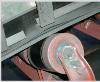
Scalloping Grooves can be created along the entire length of the belt under the skirt.
