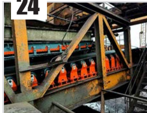
Martin Engineering: Sealed and Delivered: External Skirting Mitigates Dust, Spillage and Downtime
