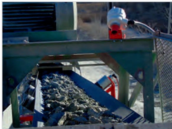
A cargo monitor can provide real-time performance data & communicate with other equipment.
