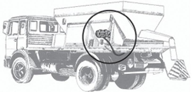
*Cougar® MDC12-400/700 vibrators improve material flow in pump trucks, spreaders and volumetric mixer trucks.*
