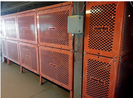
All photos copyright Martin Engineering 2023 Martin® Guarding is designed to protect workers from reach-in injuries in unauthorized areas.
