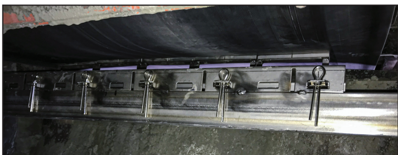
The unique stainless steel design incorporates a matrix of spring-loaded carbide tips.
