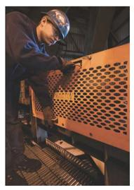
for maintenance workers. Our N2<sup>®</sup> Position Indicator technology allows our service technicians and facility managers to monitor belt cleaner wear life and tension. This significantly reduces the time spent doing regular belt cleaner inspections and provides a more predictable service schedule.
