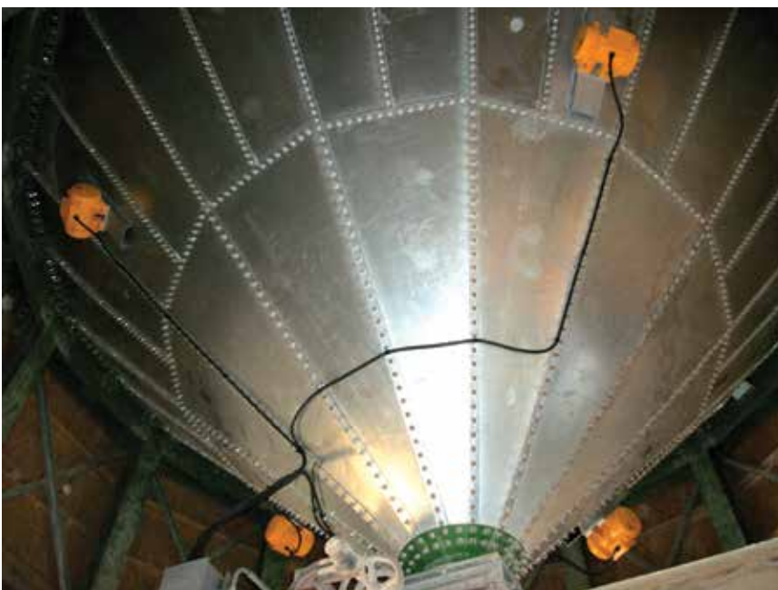
Industrial vibrators for bin & chute applications can reduce or even eliminate the need for cleaning.
