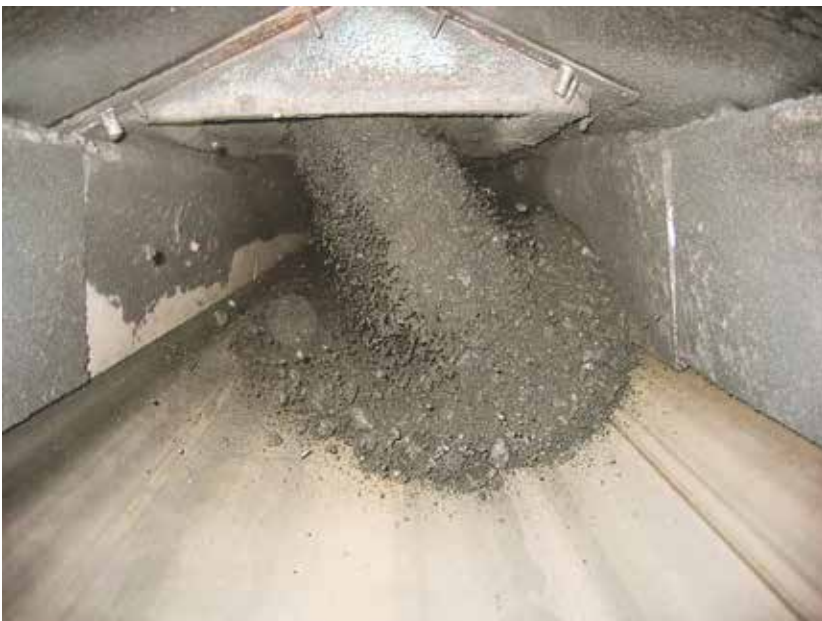
Off-centered loading puts constant abrasive pressure on one side of the loading zone causing uneven wear and mistracking.
