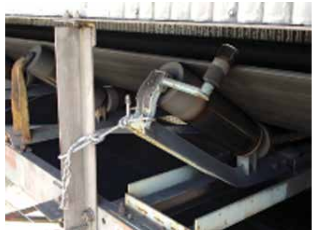
A tracking idler tied off to limit its travel.
