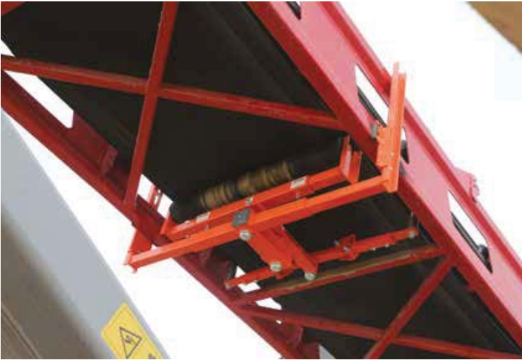
The Roller Tracker centers the cargo, reduces spillage and increases safety
