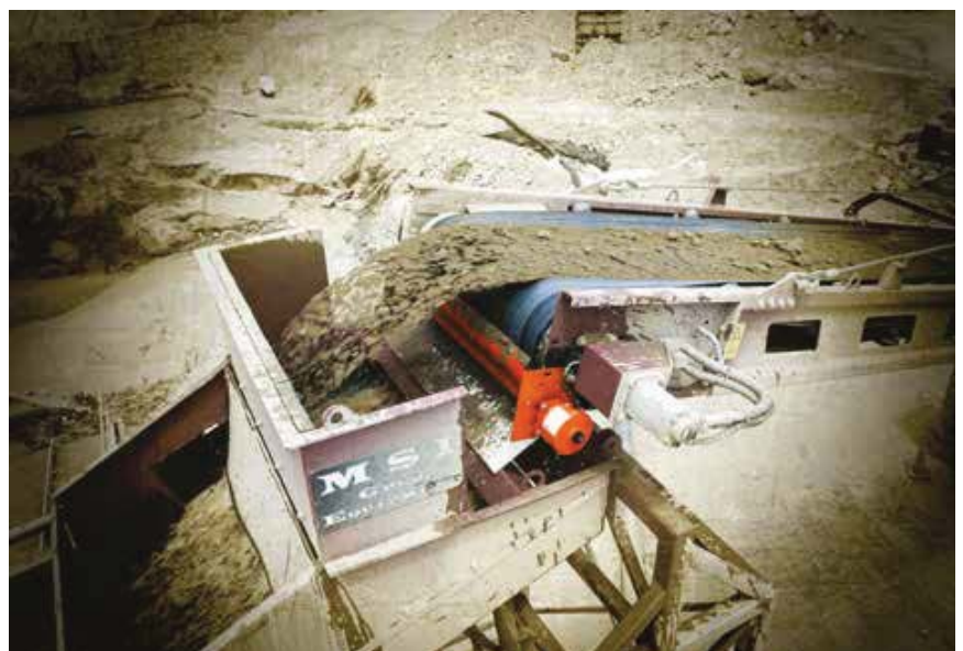
The V-Plow protects the tail pulley and belt from fugitive material on the return side.
