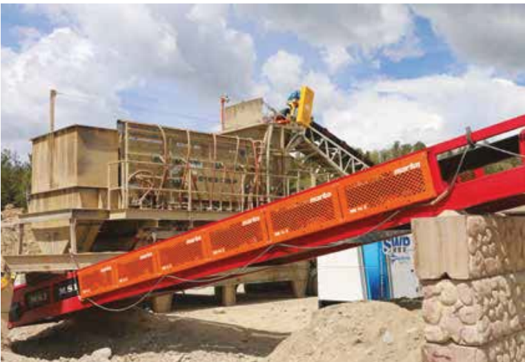
Modular conveyor guards protect workers from pinch points and other hazards
