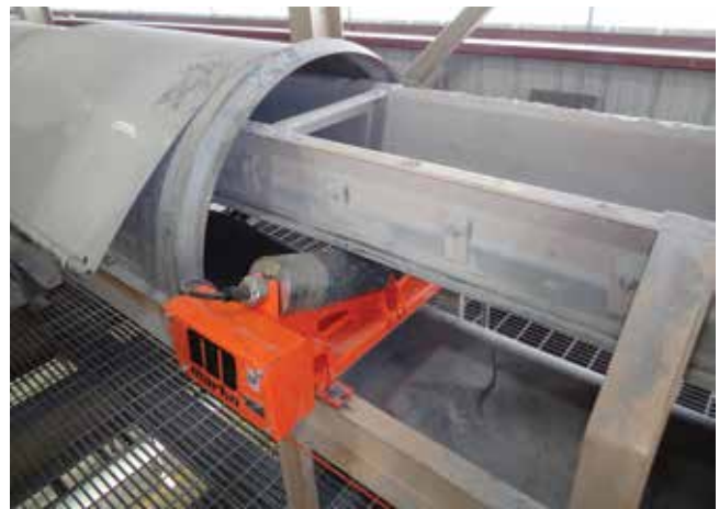
A single Roll Generator has enough power output to run a variety of accessories.
