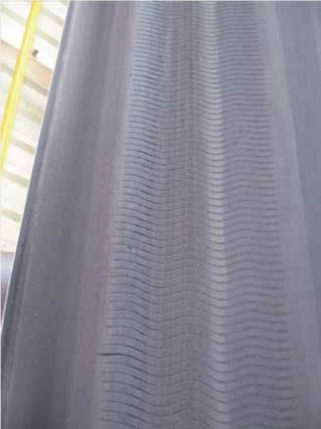
Figure 17: Positive rake / loose blade chatter marks.
