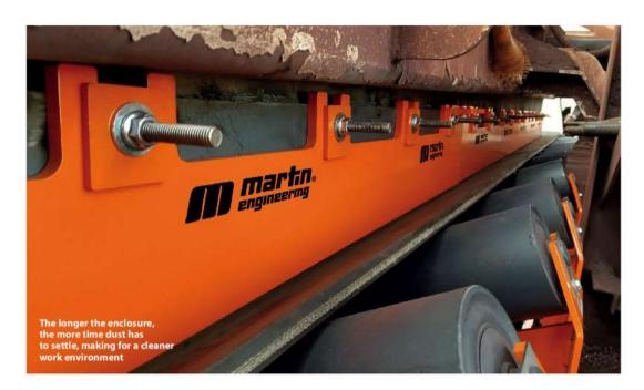
seal and clamping arrangement. With an engineered approach the height of the skirtboards is based on keeping the air speed in the enclosure below 1.0m/s. At this air speed, most nuisance dust will settle in the enclosure. When taking this approach, the quantity of air flowing through the enclosure is estimated by considering the displaced air from the initial loading, the induced air created by
