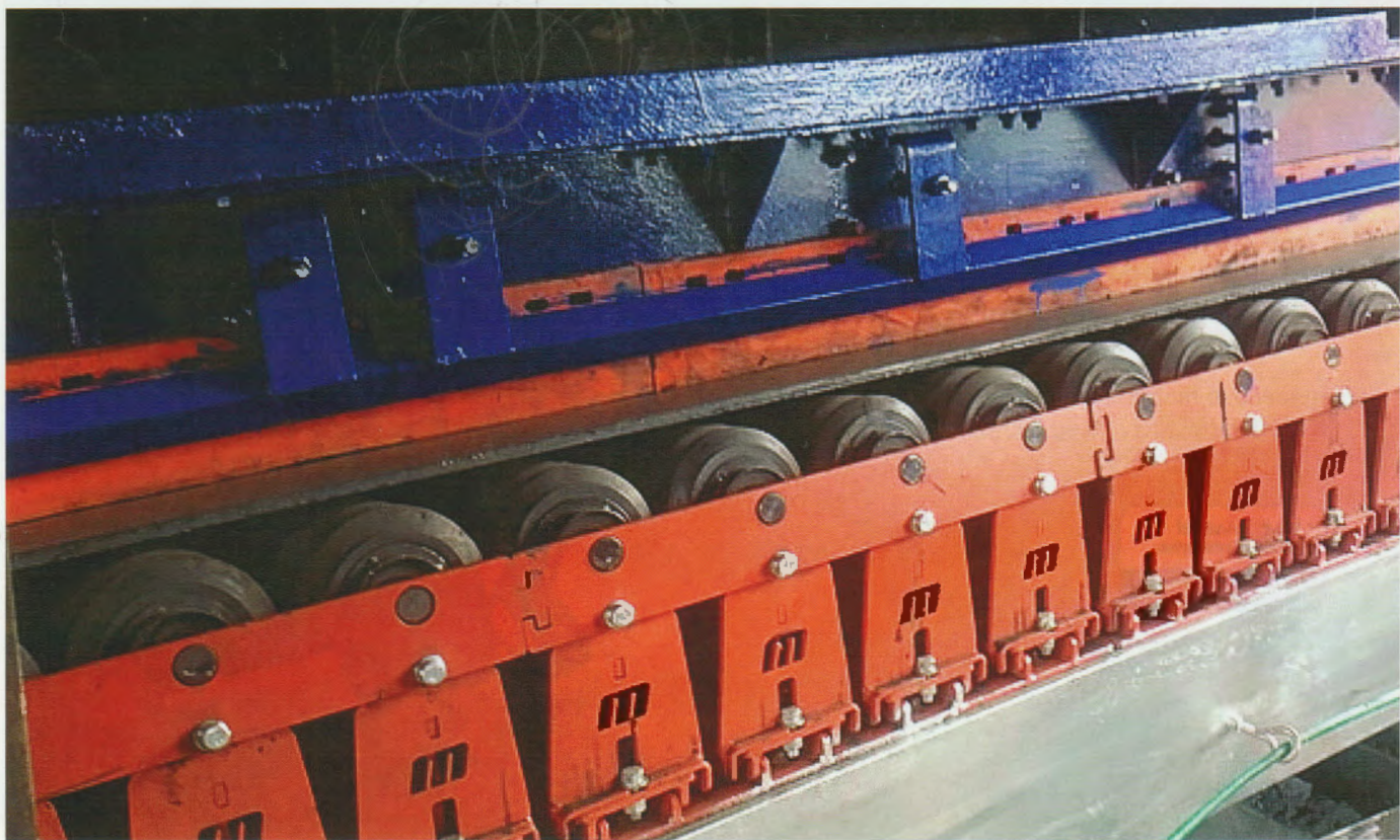
Martin Engineering's high-speed cradle helps reduce spillage
