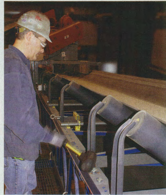
"Knocking" an idler with a mallet to change its position
