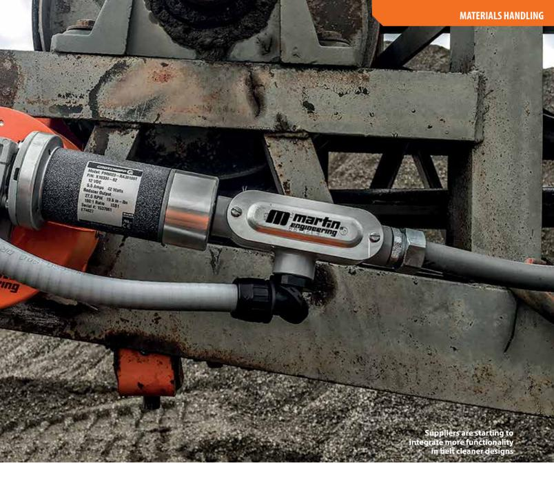
cleaner installation; there must be access to the far side for adjustment; the guide mechanisms are subject to fouling from dust and corrosion; and changing from bottom adjustment to top adjustment or providing for adjustment from one side complicates the tensioner design.
