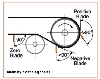
at various angles to the belt. Depending on the cleaner type and materials of construction, they can approach the belt at either a positive, negative or zero rake.
