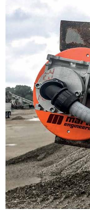
located in the secondary cleaning position or with brush cleaners. The basic tensioner design approach is typically a carriage that constrains the support frame but allows linear movement along a guide or guides roughly perpendicular to the belt surface, with the support frame and blade design providing the cleaning angle. Some designs incorporate a relief ability for impact by splices or belt defects.
