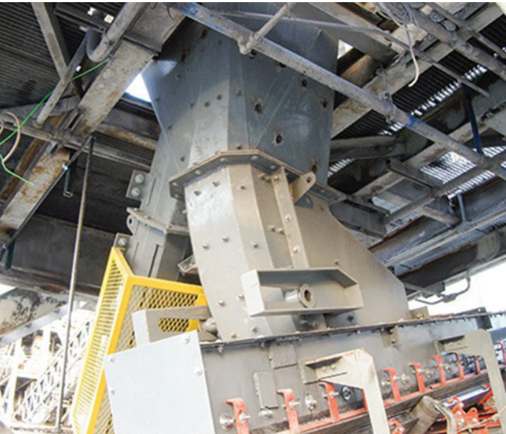
The back wall of this chute is bolted onto the side flanges, allowing the chute to be opened without confined space entry. (photo © Copyright Martin Engineering 2022)
