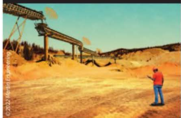
Employees and service technicians can quickly access information on networked belt cleaners via mobile phone
