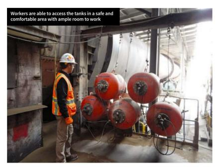
air system and weighing approximately 59kg (130lbs) each, the Martin cannons supply more force output with less air consumption at half the size of other designs. Each unit fires a shot of air at up to 8.27bar (120psi) from a pressurised tank through the long pipes and spreads the airstream across the area of build-up.
