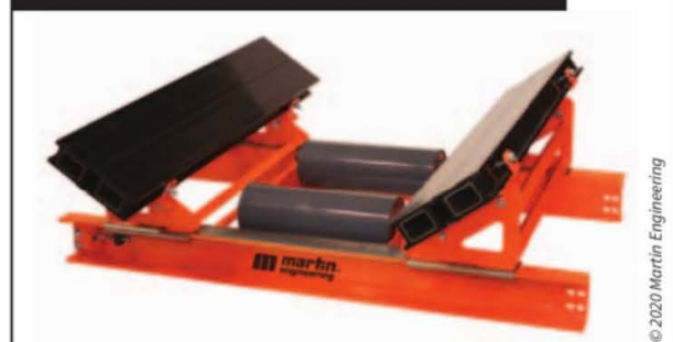
Figure 10: a "combination cradle" uses bars for sealing the belt edge and rollers to support the centre
