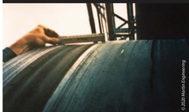
Figure 3: a groove in the belt cover can usually be attributed to entrapped material
