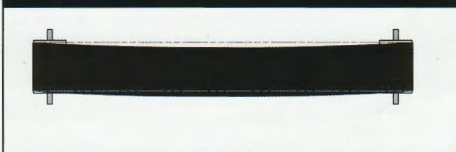
Figure 1: camber happens in the manufacturing process, and belts should be inspected prior to installation
