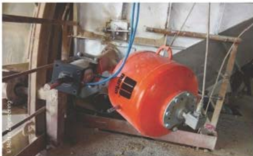
Two 70l Martin Engineering Typhoon air cannons installed at Chittor Cement, India. On the right, an air cannon fitted with a retractable nozzle
