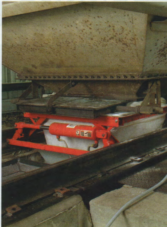
"Hammer rash" will actually worsen the problem that hammering was intended to overcome.
