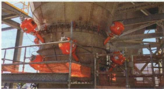
Air cannons are configured at a specific angle to enhance material flow.
