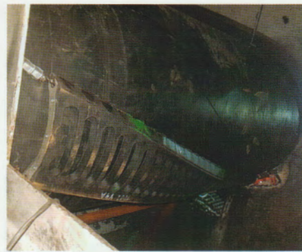
THE CLEANSCAPE RUNS NEARLY THE ENTIRE WIDTH OF THE BELT AND PULLEY
