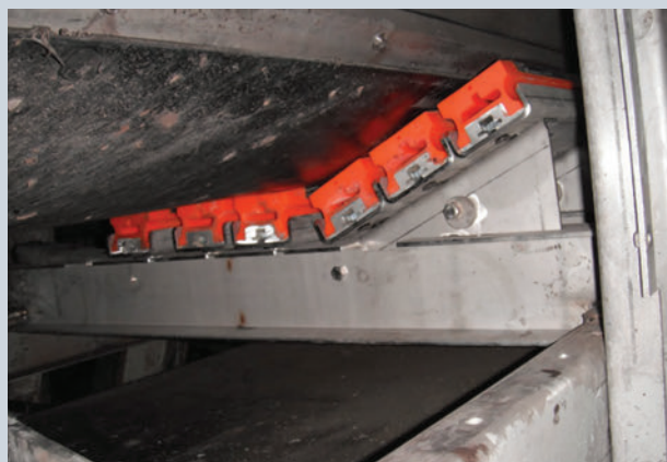
Martin's Impact Cradle absorbs the force of falling materials and objects to prevent damage to the belt and structure and eliminates any belt sag. Copyright © 2023 Martin Engineering
