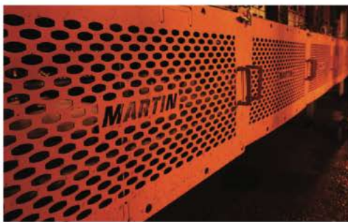
Conveyor guarding may seem like additional cost, but injury statistics make it an essential component. ©Martin Engineering 2023
