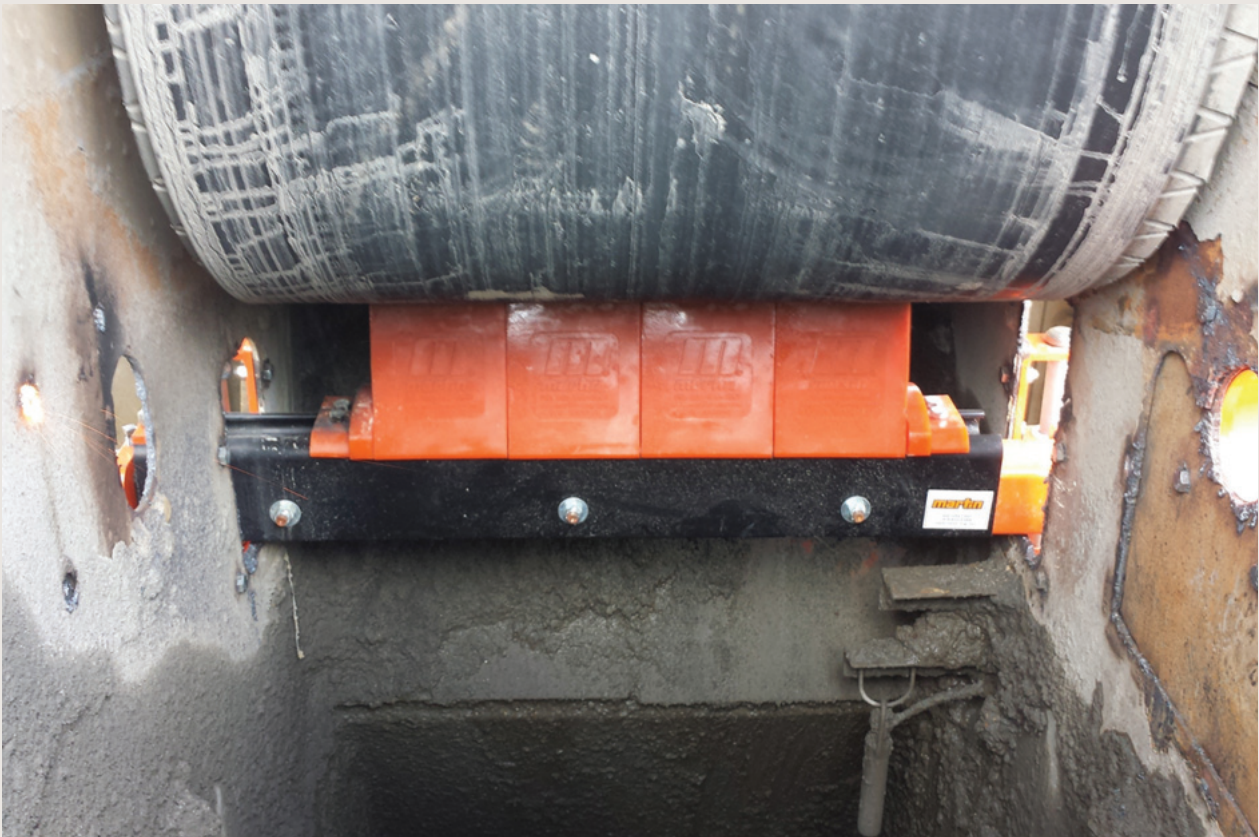
At PVDC, Martin Engineering replaced primary and secondary belt cleaners at 16 discharge points. Copyright © 2022 Martin Engineering
