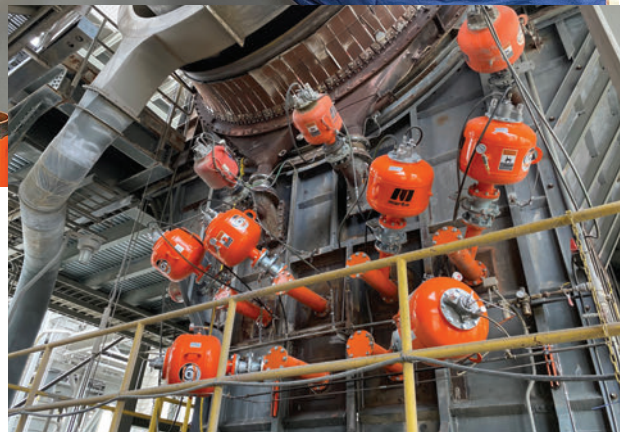
Air Cannons like Martin's Hurricane are in widespread use around the world in industries such as cement, steel, lime, coal, biomass, fertilizer and more.
