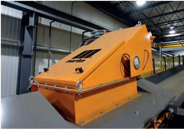
Figure 3. Mechanical air cleaners are low maintenance and improve the air quality around the system.
