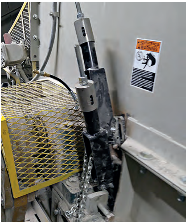
Figure 5. No tensioner monitoring or adjustment means less maintenance time, lowering maintenance costs.
