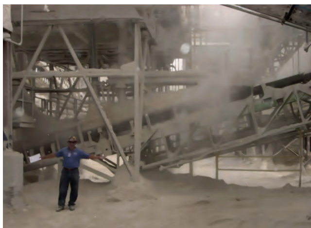
Figure 1. Dust cascading down from belt returns is a clear sign of inadequate belt cleaning.
