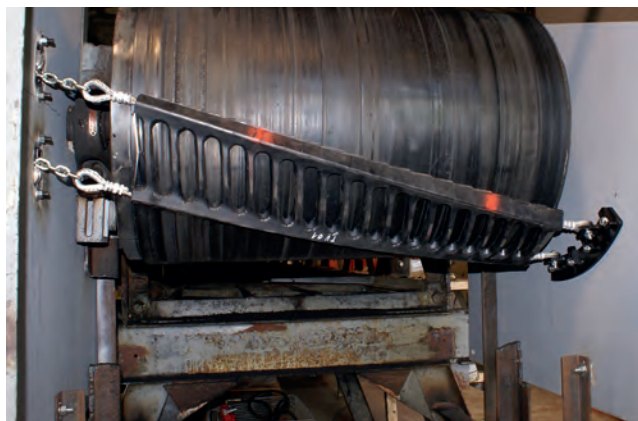
Figure 4. This innovative cleaner takes up less room and requires less maintenance than standard cleaners.
