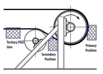
to reduce the carryback to a safe, acceptable level while limiting manual cleanup to weekly or even
