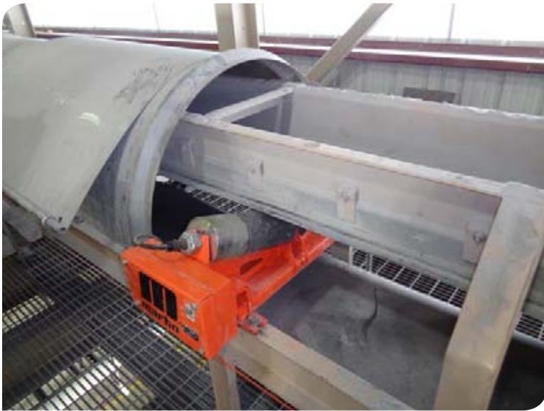
Above - Figure 4: A single Roll Generator has enough power output to run a variety of accessories.
