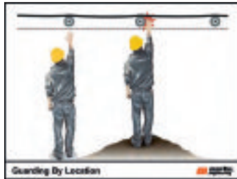
Height prevents a worker from reaching hazardous areas until the reality of bulk operations proves otherwise.
