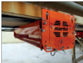
Return roller guards ensure detached rollers don’t pose a hazard to workers or harm the system.
