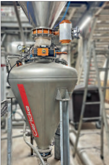
Handling cocoa powder can be tricky, due to the nature and the fineness of the powder. Gericke has supplied, installed and commissioned a pneumatic conveying, storage, feeding and mixing system for the production of chocolate drinks (see p3).
