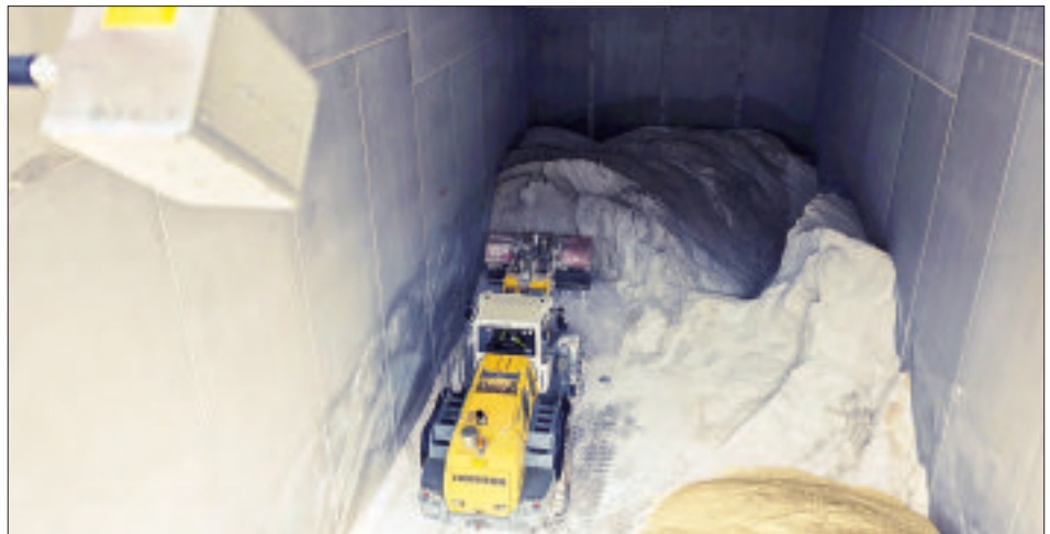
Owl Eye provides real-time volume measurement and management of bulk solids stockpiles. Data is saved in the digital platform and offers analysis functions, such as batch splitting and inventory taking (see p10).
