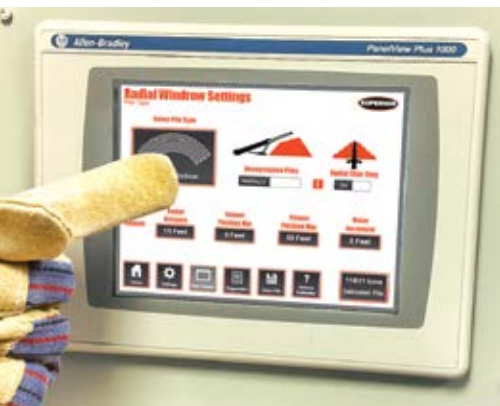
Programming PilePro Automation on a TeleStacker Conveyor requires minimal information, such as the maximum clockwise or counterclockwise travel length and the extension height increment. (Photo: Superior Industries)
