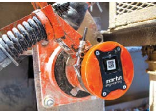
The N2 Position Indicator unit is made from rugged polyurethane, fits onto the end of the belt cleaner, is battery powered, and uses a license-exempt radio frequency. (Photo: Martin Engineering)
