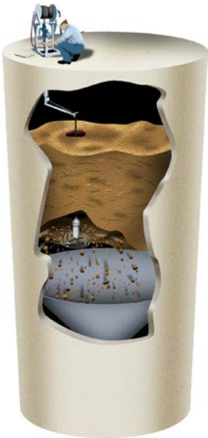
Safe, effective silo cleaning requires tools that work inside the silo from the top, controlled by personnel outside.
