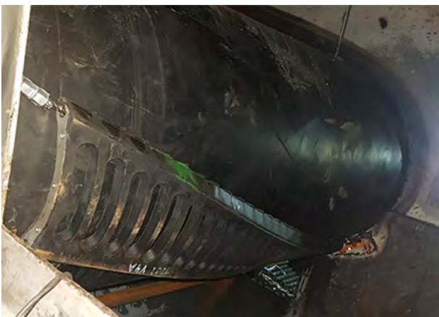
Figure 7. The low-profile CleanScrape primary cleaner takes up less space than standard cleaners.
