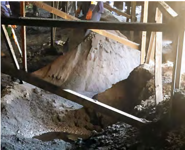
Figure 6. Spillage at the Transnet Port Terminal was pervasive, requiring regular clean-up which raised the cost of operation.
