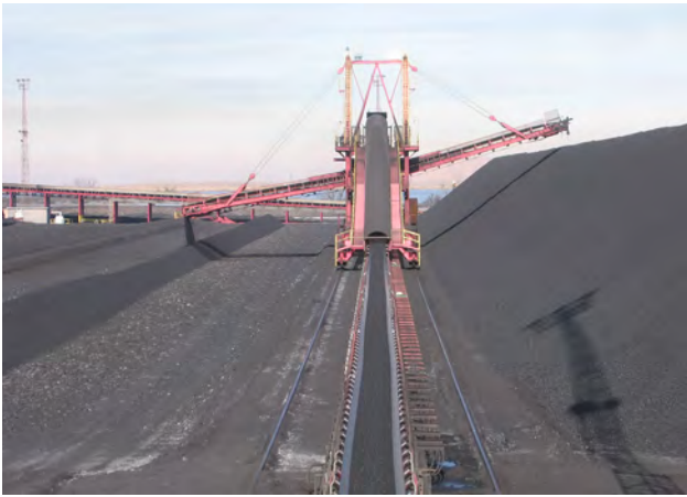
Figure 1. Port terminals of coal or petcoke with exposed stacker conveyors can be especially vulnerable to dust emissions.
