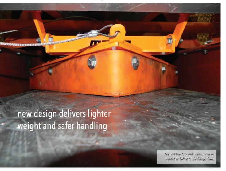
A globally respected manufacturer of bulk handling conveyor accessories has redesigned one of its most popular tail protection devices to be a lighter weight, modular unit delivered in a compact package for improved safety and convenience.
