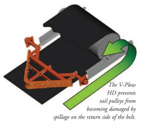
durometer nitrile rubber or long-wearing 90 Shore A durometer urethane and can be ordered with specialized blades that are chemical resistant or designed for high temperature applications.
