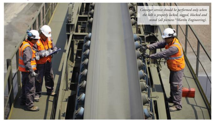
Because of their size, speed and highhorsepower drive motors, conveyors pose a number of risks to personnel working on or near them. In addition to all of the physical danger zones, when an injury occurs 'fault' is often attributed to injured workers' actions or inactions. However, safety experts point out that injuries generally occur due to a series of factors.
