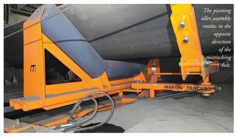
upper unit before the discharge, operators ensure the belt is centred on the head pulley allowing for optimal belt cleaning with maximum cargo discharge.
