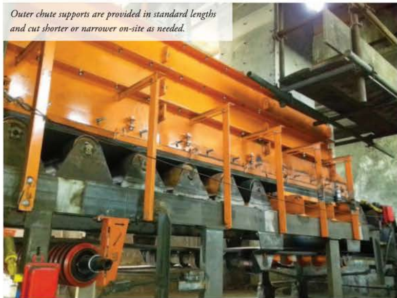
The Transfer Point Kit can be assembled prior to installation or assembled during scheduled downtime.
